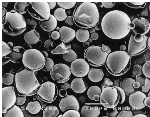
Figure 1 SEM image of POE8 microparticles prepared using POE8 (50 mg/mL in DCM) and 0.01 w/v % PVA stabilizer concentration (bar size = 100 \mu\text{m} ).
